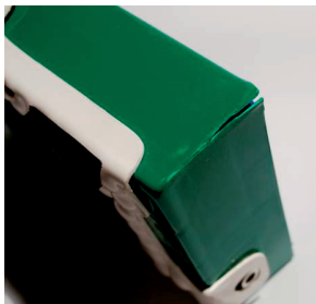
Figure 7.2 - The Bricket case began to crack over time.
